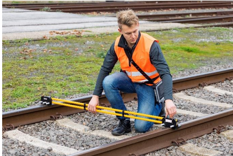
Applying the gage
