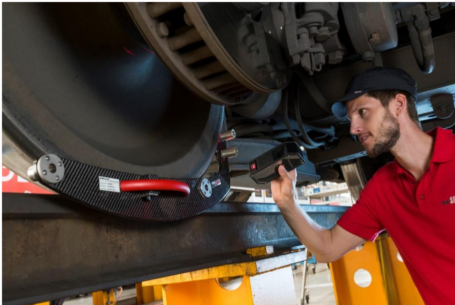
Wheel Diameter measurement with sensor and D-Gauge
