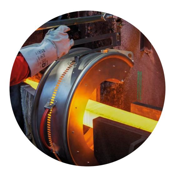
To optimise the rolling process and set the optimum rolling parameters, roll pass designers have always had to adopt inaccurate and time-consuming processes – until now! CALIPRI delivers reliable measured data between passes and on profiles that are still hot in a way that is both efficient and accurate.
